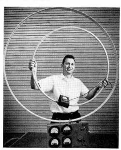
HULA HOOP WITH A FUTURE: Amado Chavez (7333) decided a hula hoop would meet specifications for a semi-rigid, nonconductive covering for the wires of a transmitting antenna. The more conventional prototype is in the foreground.
